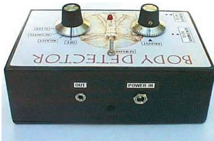
Rear view of the completed Body Detector showing the power input socket and output socket. The author also drilled a hole between the sockets for the insertion of a thermometer. Note the sensor bolt on the top of the case.
