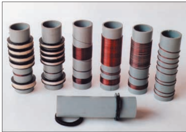
Tuning coils for radio receivers: These hand-wound coils are illustrated in Fig.1, and details of the windings are given in Table 1 and Table 3. The card bobbins for the pie-windings have been dipped in black cellulose to stiffen them.
