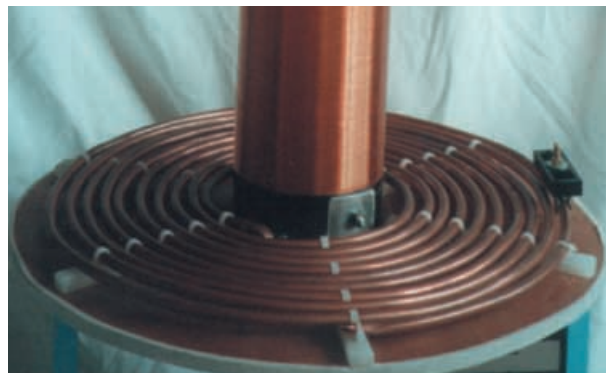
Assembled primary coil and its base board. The secondary coil is seen in the centre. Note the tapping clamp at the right.
