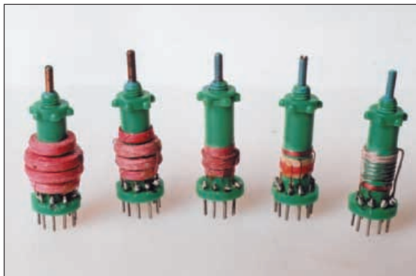
Tuning coils: Machine-wound coils on 9mm diameter ferrite cores. Five coils together with a 10pF to 330pF tuning capacitor cover 150kHz to 30MHz. Originally manufactured by Denco, we understand they are no longer in production.
