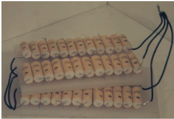
Secondary coil's capacitor (C2) assembly.
