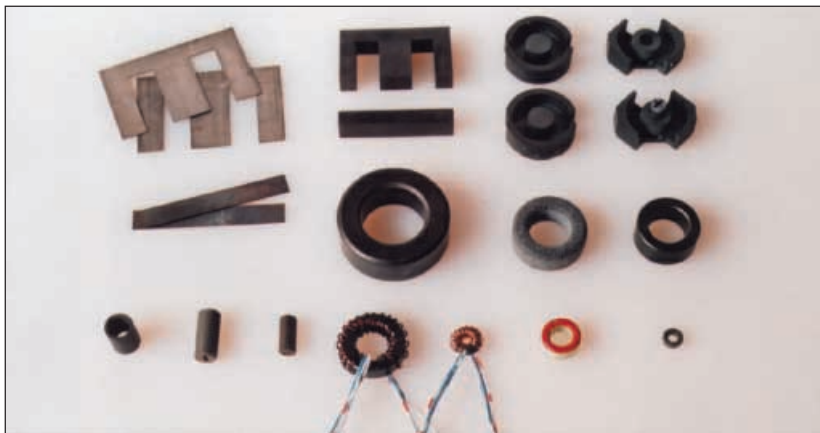
Core materials: Soft iron "E" and "I" laminations, a dust iron "E" and "I" moulding, ferrite pot core assemblies, ferrite and dust iron toroids, dust iron threaded cores: different materials for different frequencies. The wound toroids are large and small versions of the broadband transformer illustrated in Fig.6.
