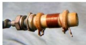
Adjustable air-wound inductor
